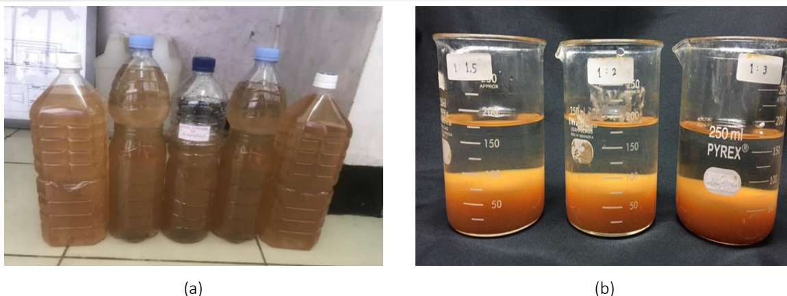
Figure 3. Color of Pharmaceutical Wastewater (a) Before, (b) After Treatment of Photo-Fenton Process
